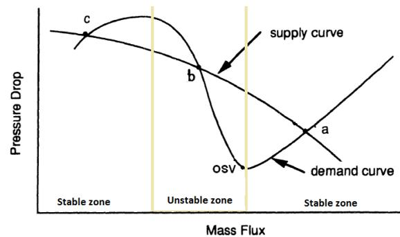
Fig. 3 – Natural circulation stable and instable operating zones.
