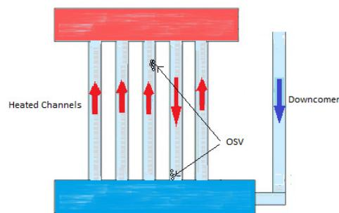
Fig. 4 – Possible NC flow under spent fuel pool storage conditions
