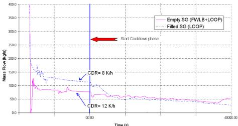
Fig. 2 – Low cooldown rate maintaining natural circulation during asymmetric cooldown.
