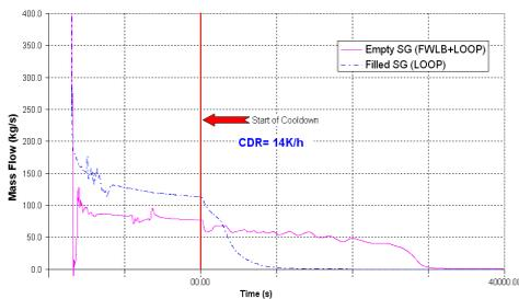
Fig. 1 – Natural circulation Interruption during asymmetric cooldown
